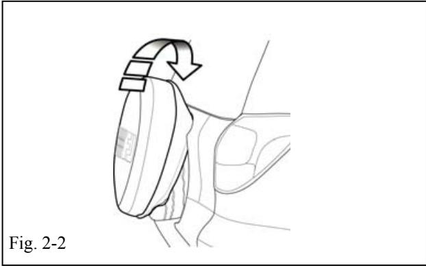
(c) Start by slipping the top half of the soft vinyl part of the cover completely over the top of the tire (Fig. 2-2.)
