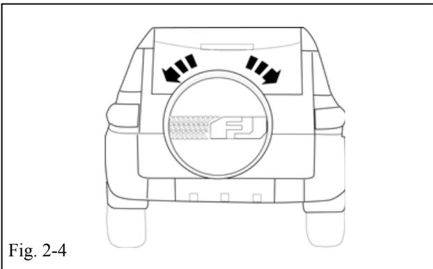
(e) Once all the vinyl has been installed as far as possible, manually spin the cover while pressing inward to fully seat the remainder of the vinyl. (Fig. 2-4)
