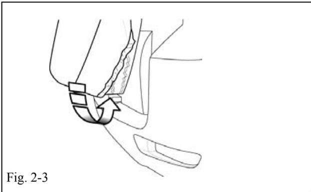
(d) To install the bottom half, open the back door to gain access to the bottom of the tire.
